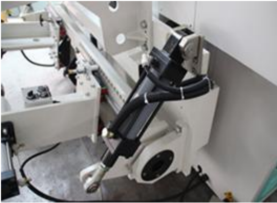
Unwinding Hydraulic Lifting
